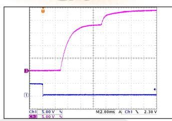
Figure 7: Typical startup waveform. Input voltage pre-applied, ON/OFF Pin on Ch 1.
