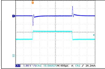
Figure 11: Output voltage response to step-change in load current (50%-75%-50% of Iout(max);  $dI/dt = 0.1 A/\mu s$ ). Load cap:  $I \mu F$  ceramic and  $I5 \mu F$  tantalum capacitors. Ch 1: Vout (IV/div), Ch 2: Iout (IV/div).
