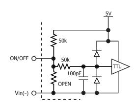
Figure B: Internal ON/OFF pin circuitry
