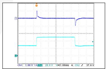
Figure 12: Output voltage response to step-change in input voltage (250V/ms). Load cap:  $100 \mu F$  electrolytic output capacitance. Ch 1: Vout (1V/div), Ch 2: Vin (20V/div).
