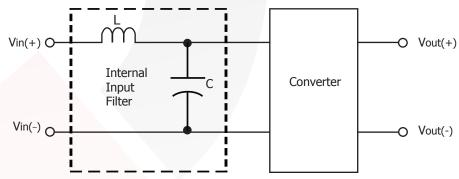
Figure E: Internal Input Filter Diagram
