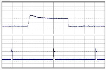
**Figure 18:** Load current (5A/div) as a function of time (2ms/div and 50ms/div) when the converter attempts to turn on into a 10 m $\Omega$  short circuit.
